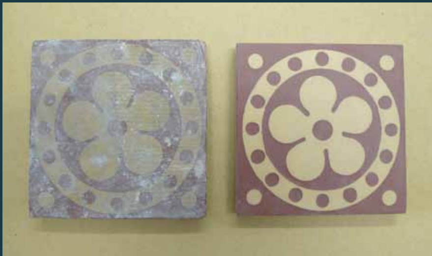
Below: Tile specialists Craven Dunnill recreated both geometric and encaustic tiles from original samples. They were carefully colour-matched. Some colours had to be specially made. The development cost of producing a replica encaustic tile is £500. Thereafter, each replica tile of the same design costs £25. £30,000 was spent to produce 15 different encaustics and 50+ different coloured and shaped geometric tiles.
