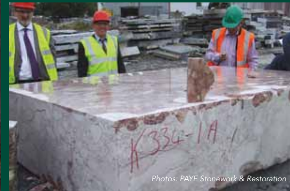
Above (both): It was difficult to find an alternative for the Cork Red limestone featured on the original screen. However, after inspecting several blocks of Kerry Red in Irish quarries, one of the correct colour was eventually found.
